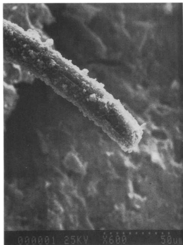
FIGURE 8. PVA fiber extending out from a fracture surface (600 \times magnification).
