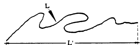
FIGURE 7. Linear roughness R_l = L/L' .
