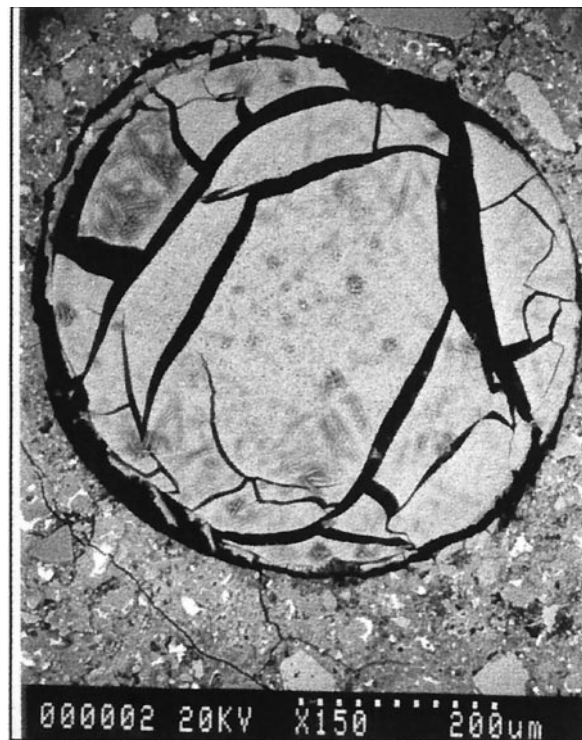
FIGURE 6. Specimen L1b (1M Na/KOH at 38°C/0% fly ash). BSE image showing air void filled with gel.
