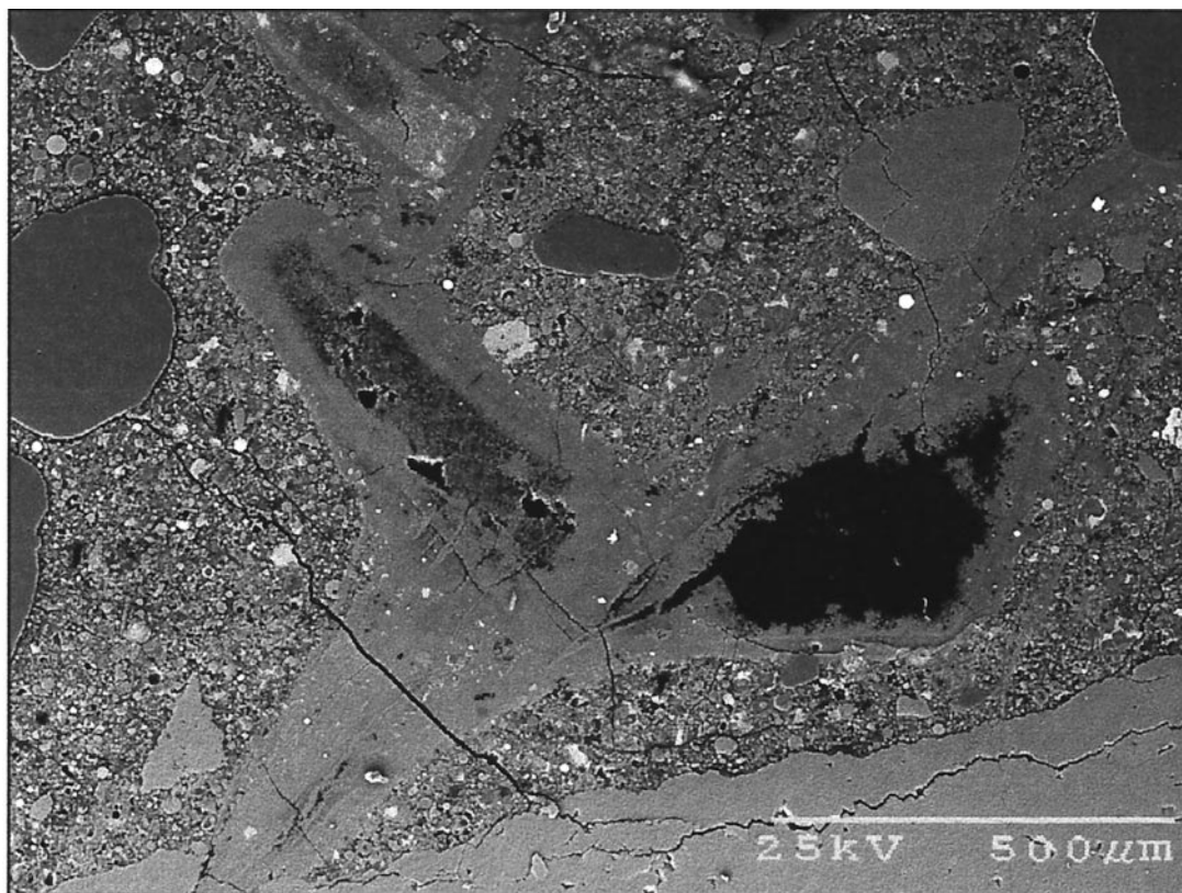
FIGURE 12. Specimen L9a (1M NaOH at 80°C/40% fly ash). BSE image showing “river” of alkali-silica gel flowing through cement paste from reacted flint particles.
