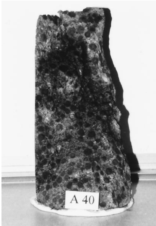
FIGURE 2. Fractured surfaces of the lightweight aggregate concrete.
