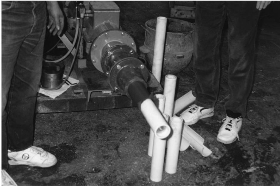
FIGURE 1. Extrusion manufacturing process for FRC pipes.
