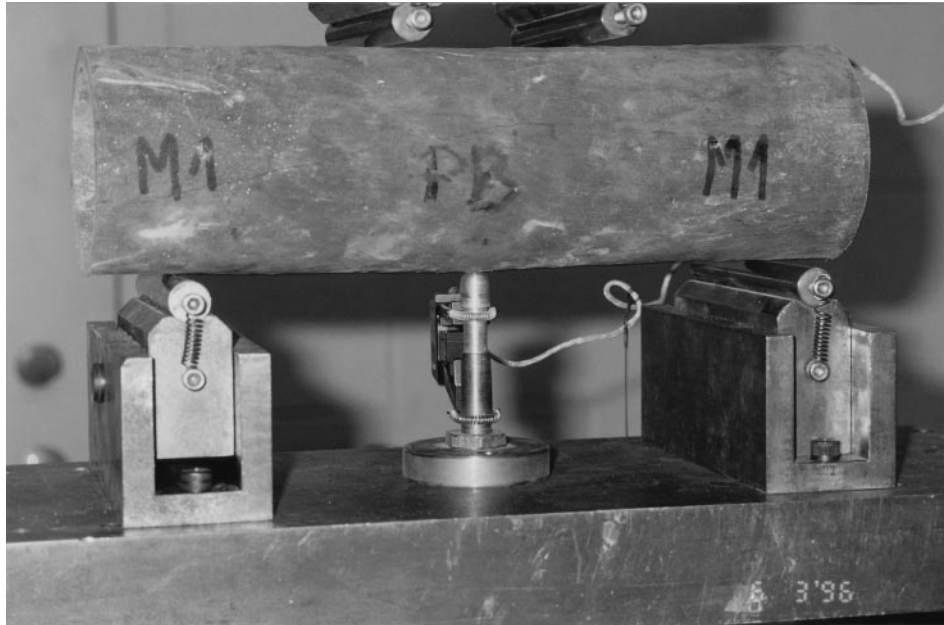
FIGURE 4. Test set-up for flexural strength of pipe and typical pipe failure.
