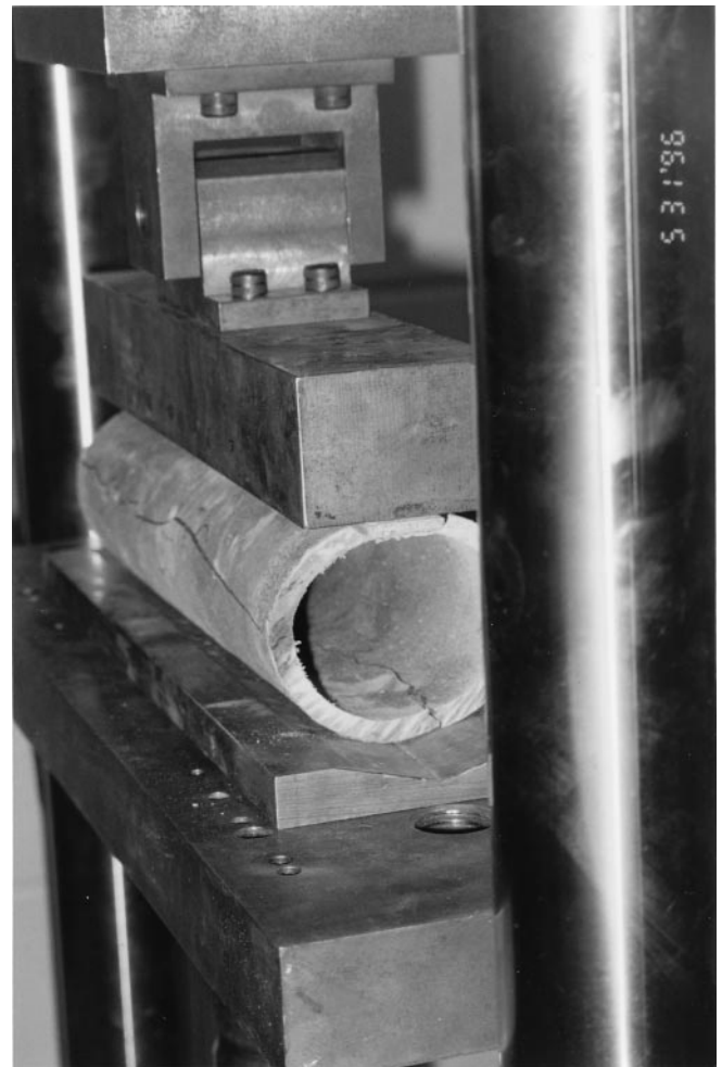
FIGURE 3. Test set-up for V-shaped three-edge bearing strength of pipe and typical crack pattern at failure.
