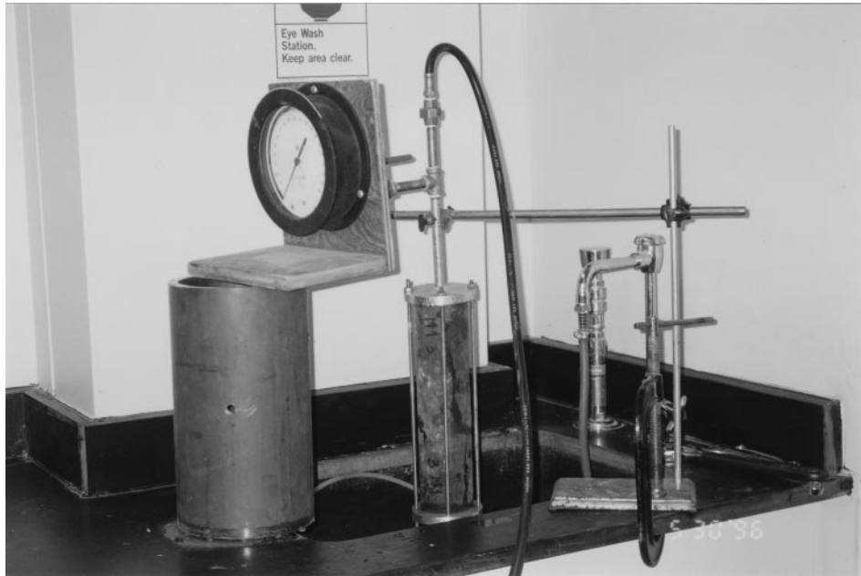
FIGURE 2. Test set-up for hydrostatic pressure/burst strength of pipe.
