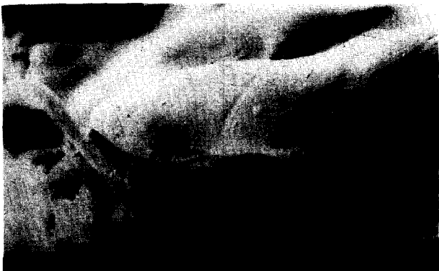
Fig. 11. SEM of fractured surface of unmodified mortar. Heterogeneity is prominent.
