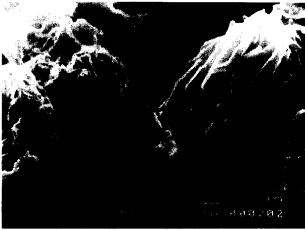
Fig. 5. High magnification of the aggregate surface at the aggregate-matrix interface in 90 days cured concrete with untreated Lytag aggregate.
