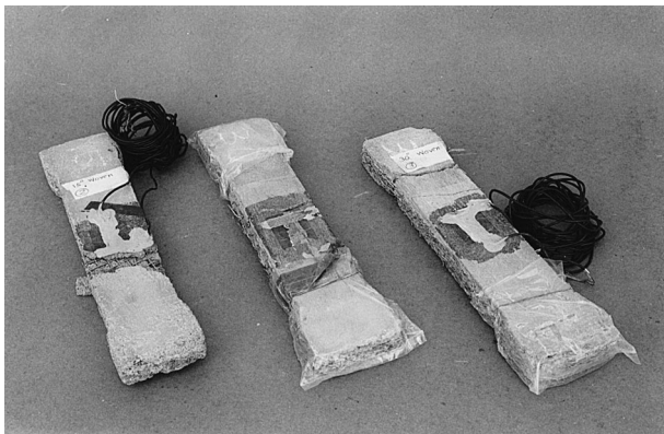
Fig. 4. Ferrocement specimens tested under in-plane tension.
