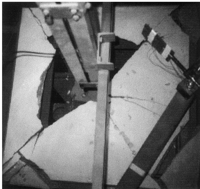
Fig. 4. Failure of plain concrete slab.
