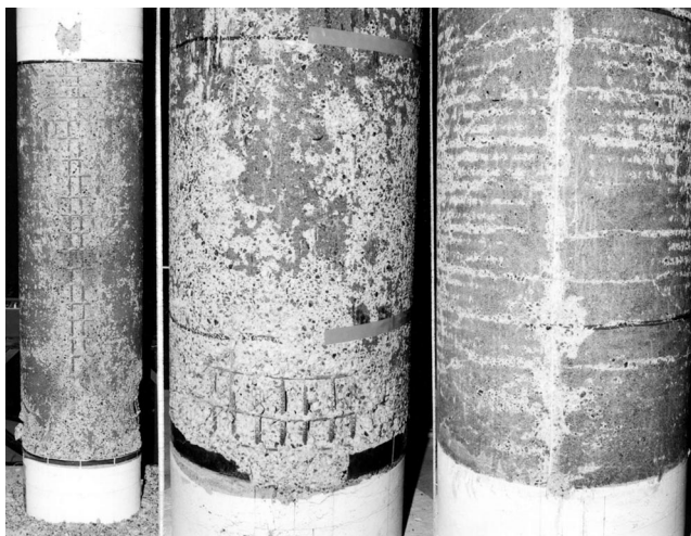
Fig. 14. Conditions after CFS were peeled off.
