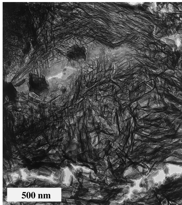
Fig. 19. Transmission electron micrograph showing foil-like Op C-S-H in a CH-slag paste hydrated for 3\frac{1}{2} yr.
