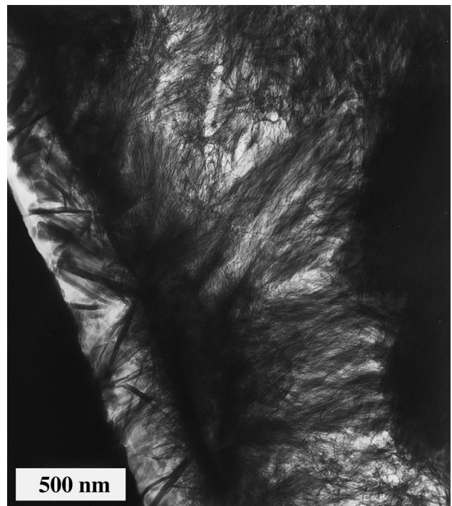
Fig. 24. Transmission electron micrograph showing a well-defined slag inner product region containing Mg, Al-rich precipitates which are oriented towards the Ip/Op interface in a 50% ordinary portland cement 50% slag paste hydrated for 1 month.
