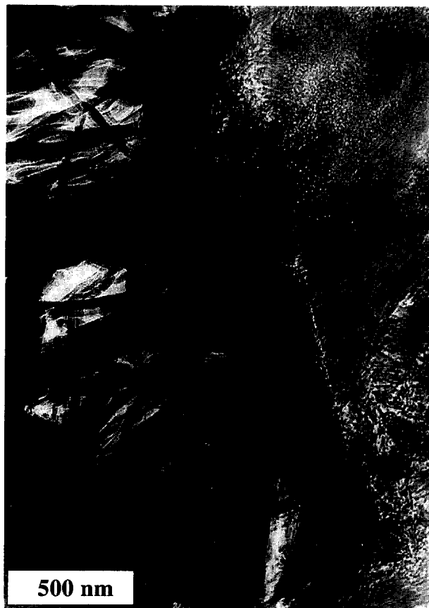
Fig. 4. Transmission electron micrograph showing coarse fibrillar Op C-S-H between two regions of synthetic slag-glass Ip in a 50% C 3 S 50% synthetic slag-glass hydrated for 1 month.
