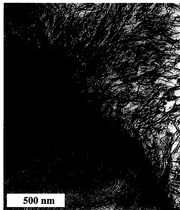
Fig. 1. Transmission electron micrograph showing a region of slag-derived Ip (bottom left) with fine dense morphology and foil-like Op C–S–H in a 90% slag 10% C 3 S blend hydrated for 18 months at 20°C.
