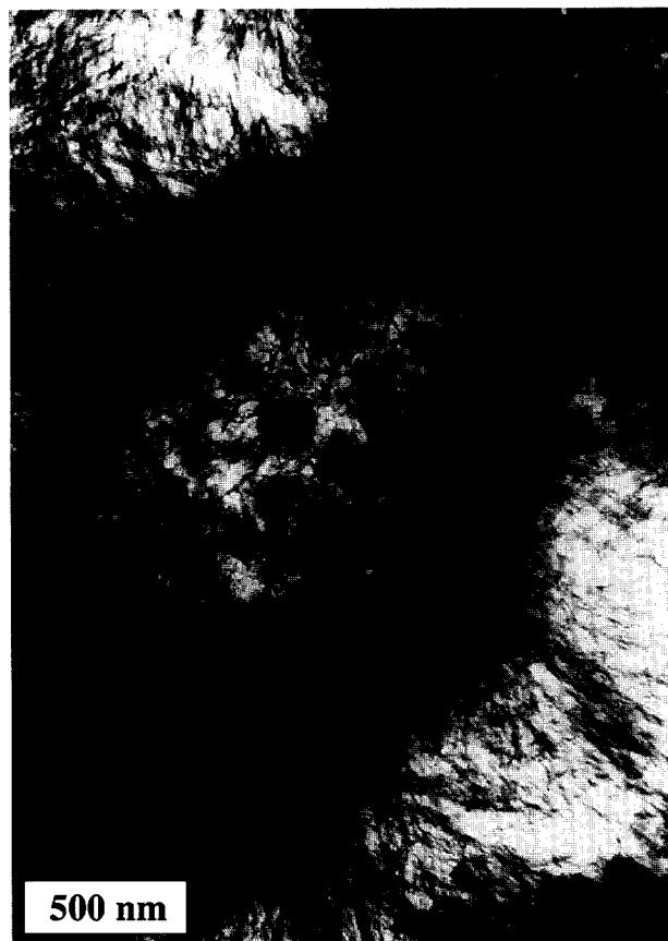
Fig. 3. Transmission electron micrograph showing two types of inner product in a 90% slag 10% C_3S blend hydrated for 18 months at 20°C: Ip from a C_3S grain (top right) and a small fully hydrated slag grain (centre-left).
