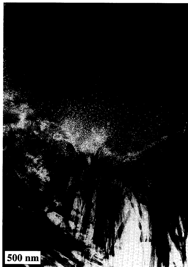
Fig. 5. Transmission electron micrograph showing coarse fibrillar Op C-S-H surrounding a partially hydrated C 3 S grain in a 50% C 3 S 50% synthetic slag-glass hydrated for 1 month.
