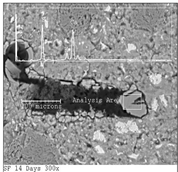
Fig. 10. X-ray spectrum of opal aggregate in sample incorporating SF taken 14 days after immersion in 1 N NaOH.
