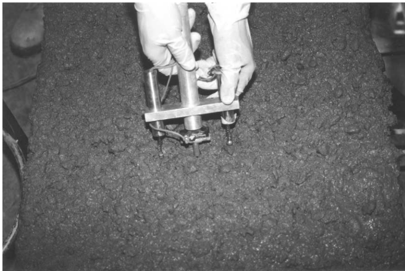
Fig. 4. Measurement of penetration resistance of shotcrete soon after placement.
