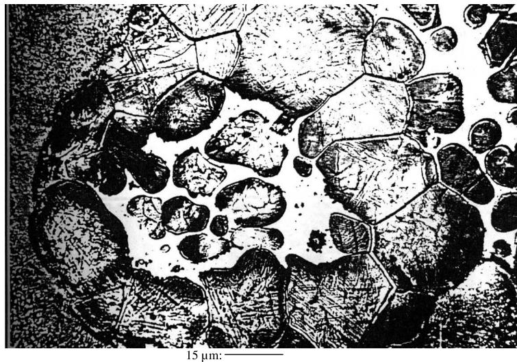
Fig. 4. Belite rosette (clayey origin).
