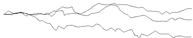
Fig. 13. Generation of three random crack patterns (crack length: 50 mm; SD of the angle: 30°; mean of the length segments: 0.5 mm; SD of the length segments: 0.25).
