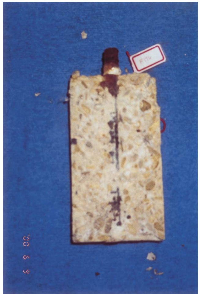
Fig. 4. Specimen made from concrete with fibers after 46 months of chloride exposure.
