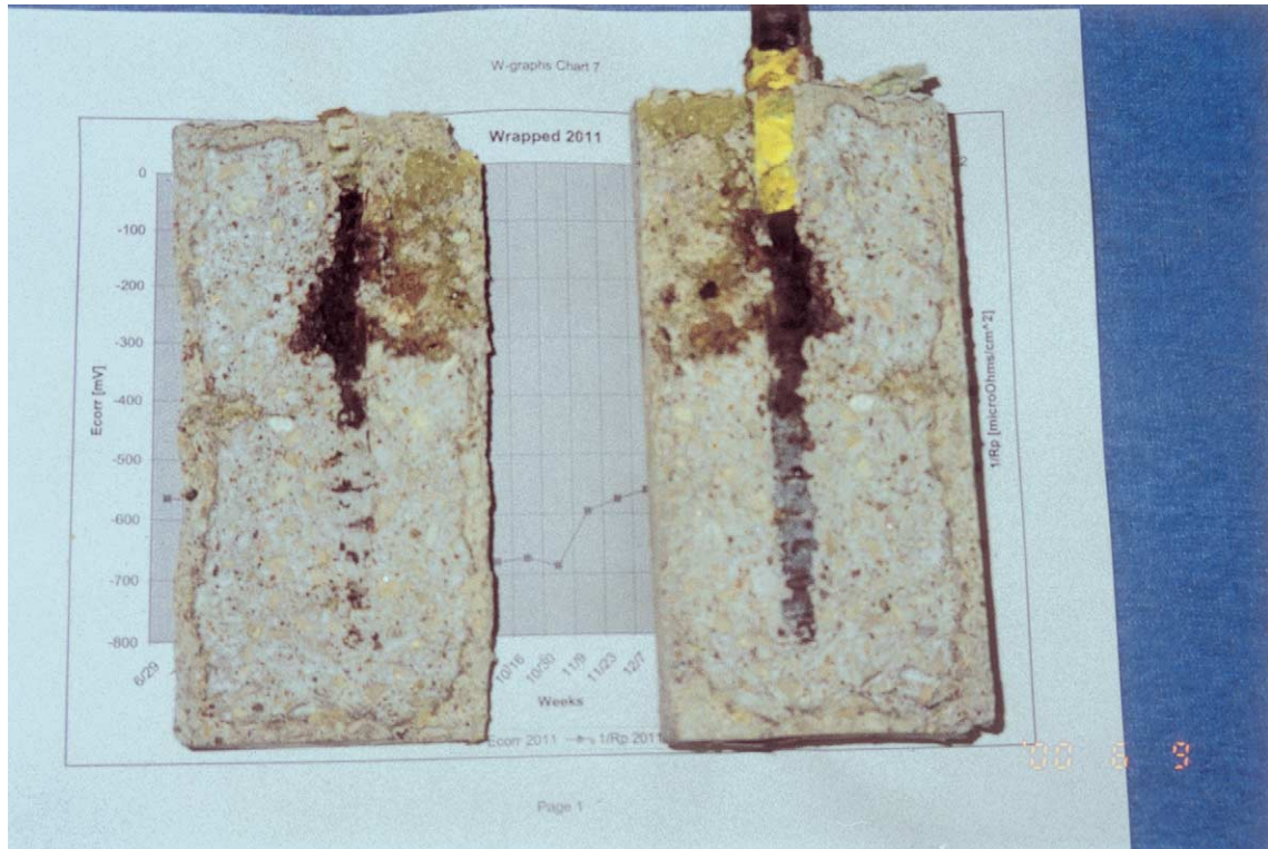
Fig. 10. Specimen made from Mix 20 after chloride exposure for 12 months, encapsulation, and re-exposure to chlorides for 22 months.
