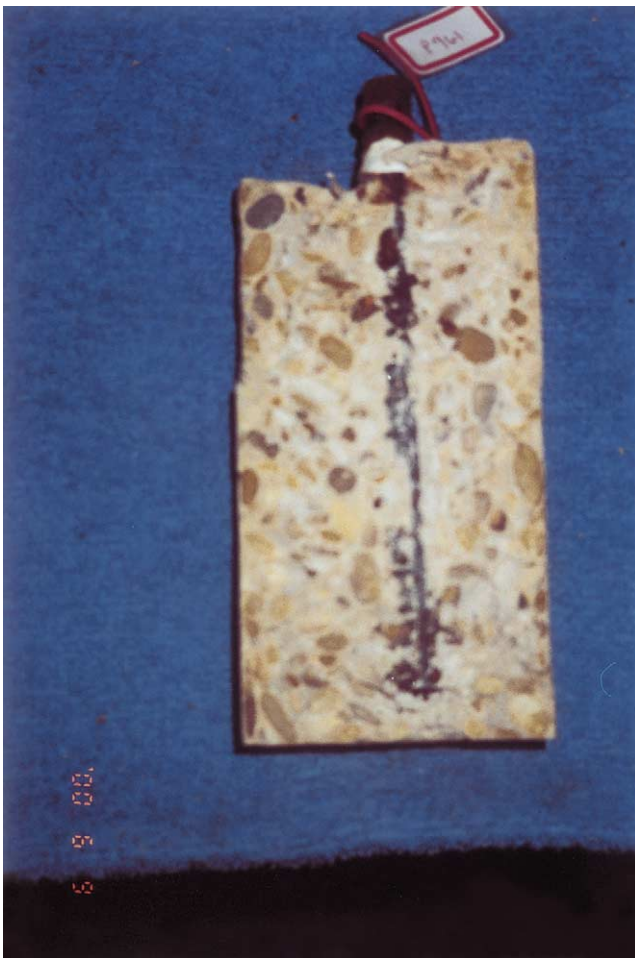
Fig. 3. Specimen made from concrete without fibers after 46 months of chloride exposure.
