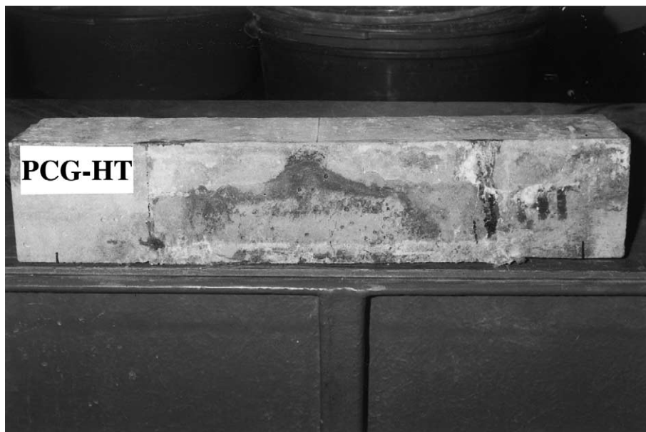
Fig. 8. PCG–HT-4 beam after accelerated reinforcement corrosion.
