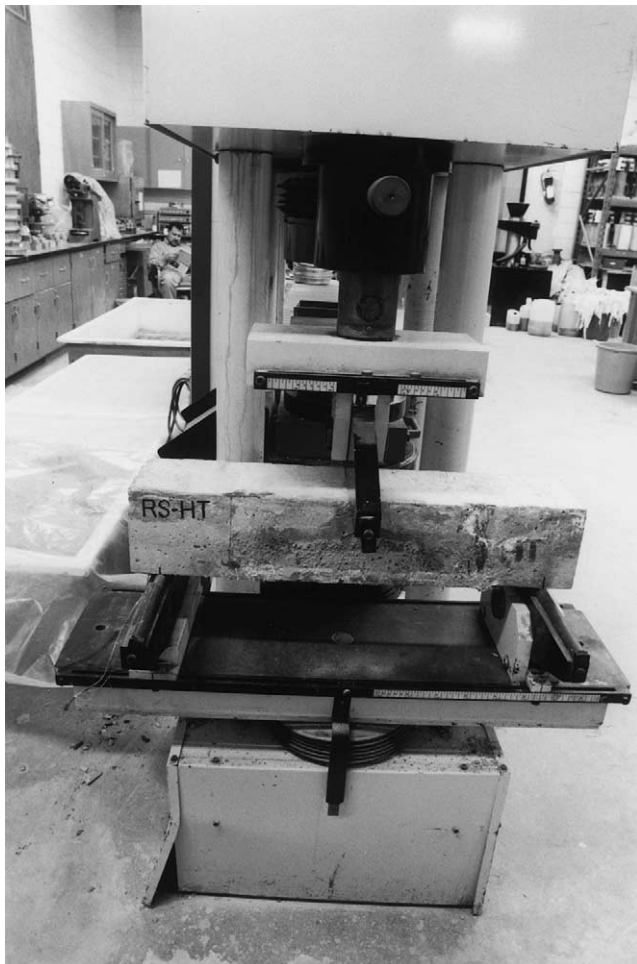
Fig. 2. Setup for determination of flexural strength.
