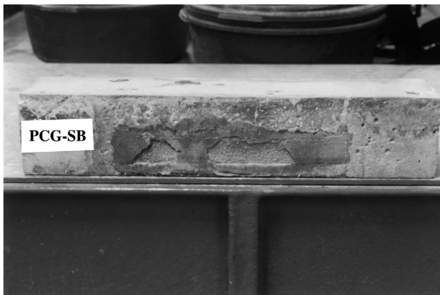
Fig. 6. PCG-SB-4 beam after accelerated reinforcement corrosion.
