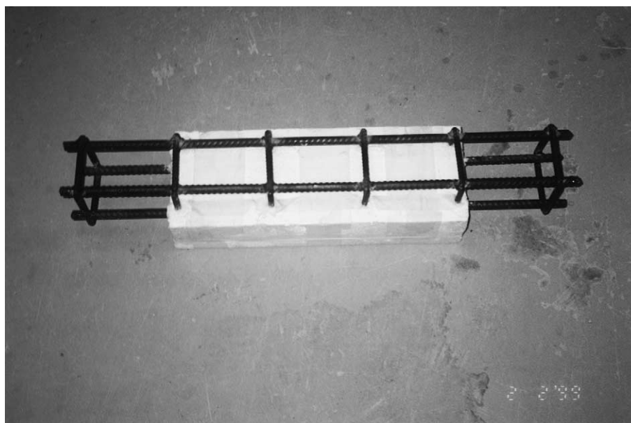
Fig. 1. Steel cage with Styrofoam before concrete casting.
