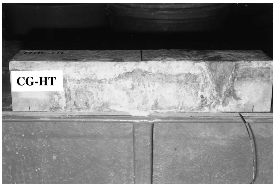
Fig. 9. CG-HT-4 beam after accelerated reinforcement corrosion.
