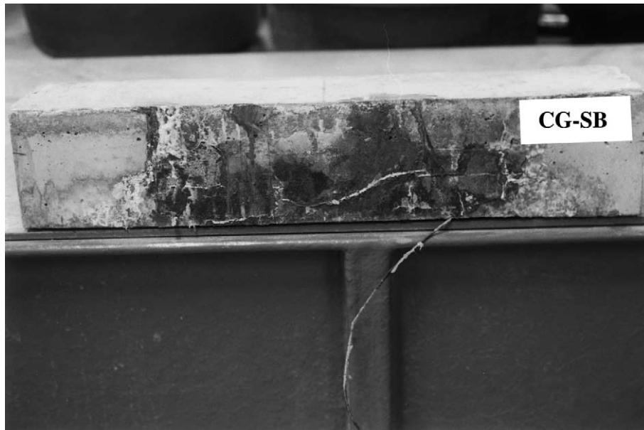
Fig. 7. CG–SB-4 beam after accelerated reinforcement corrosion.
