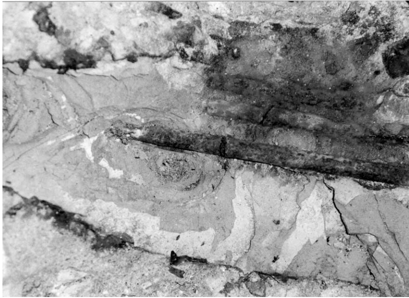
Fig. 12. Stress corrosion cracking of the prestressed wires.
