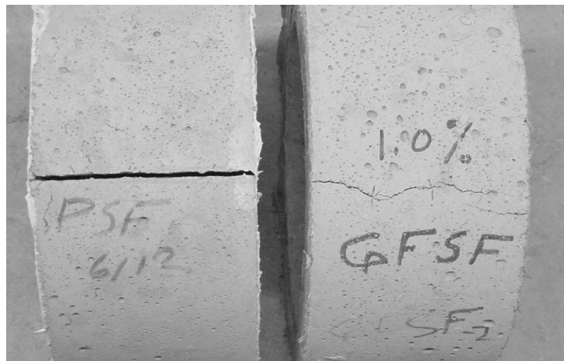
Fig. 8. Picture of plain (left) and glass fiber (right) reinforced restrained shrinkage specimens.
