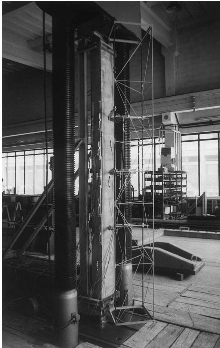
Fig. 9. Overall view of test stand. Truss construction for measuring displacements is visible.
