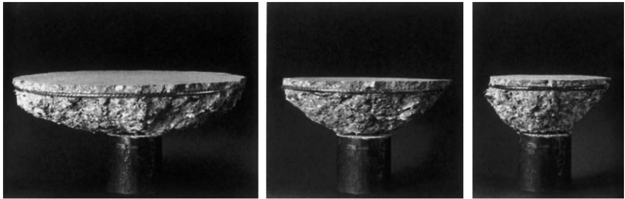
Fig. 2. Punching cone with different inclinations: 30°, 45°, and 60° [17].
