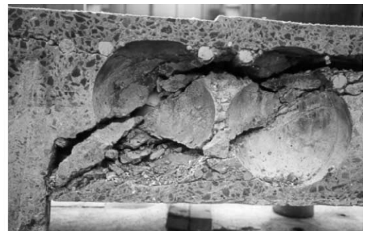
Fig. 12. Comparison of the internal crack pattern in computation and in test.
