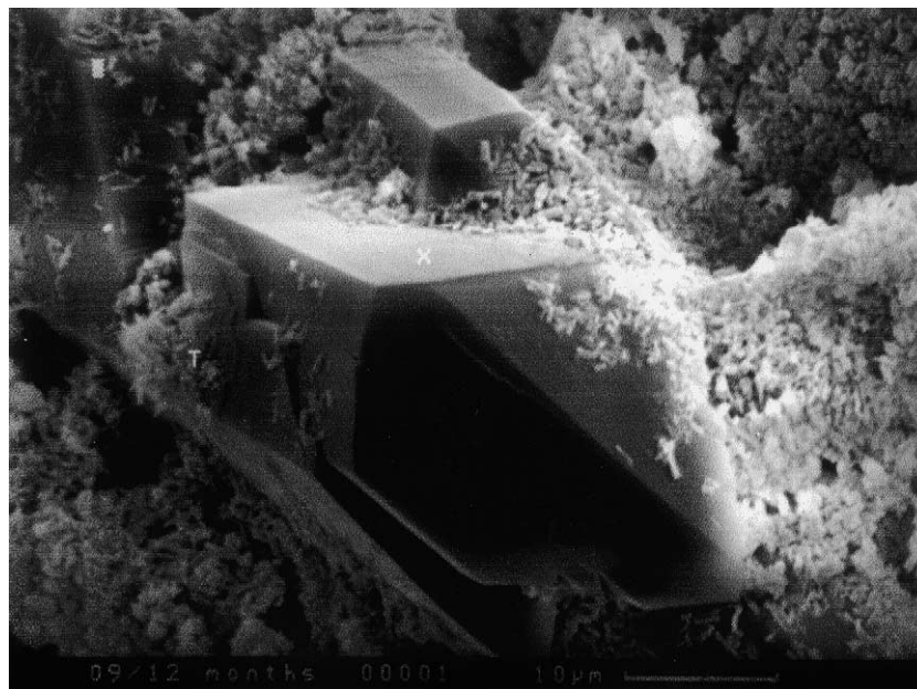
Fig. 10. Secondary electron image of the large tabular gypsum crystal surrounded by fine needles of thaumasite (T = thaumasite, X = gypsum).
