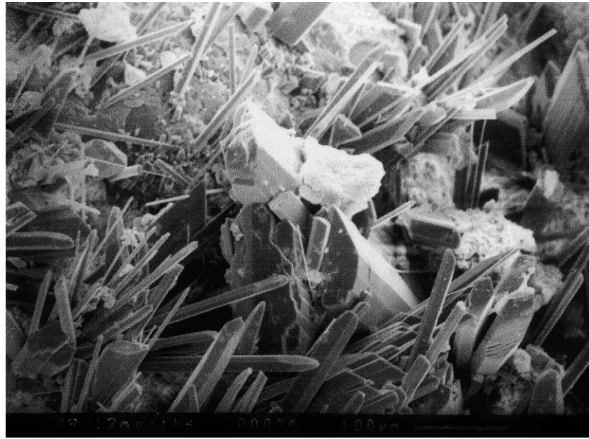
Fig. 6. Secondary electron image of a deteriorated OPC – 35% limestone cement mortar stored in 1.8% \text{MgSO}_4 solution at 5 °C for 364 days.
