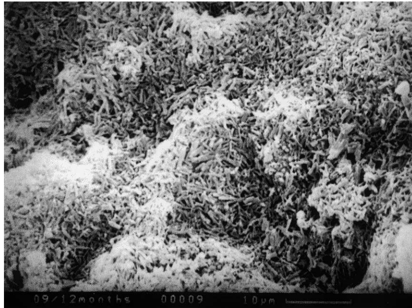
Fig. 8. Secondary electron image of the same mortar.
