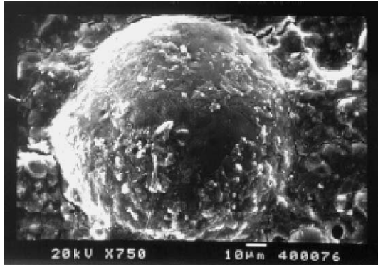
Fig. 4. Fly ash particle covered with a crust of reaction products.
