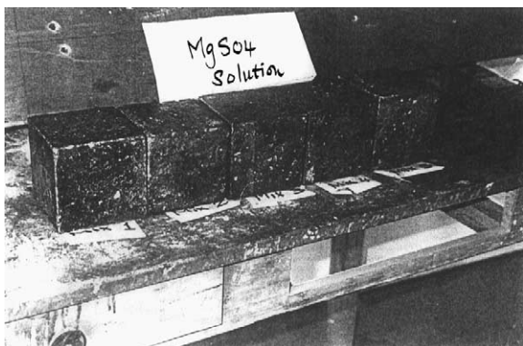
Fig. 3. Relative behavior of concrete mixes stored in MgSO 4 solution.
