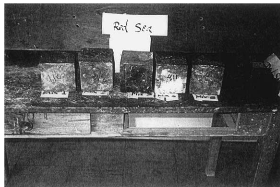
Fig. 6. Relative behavior of concrete mixes stored in Red Sea water.
