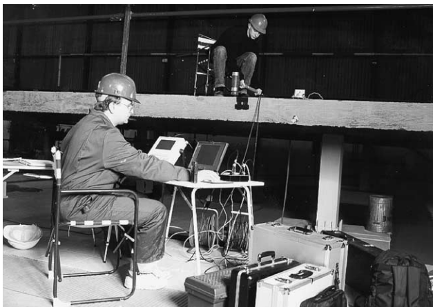
Fig. 4. Hammer excitation and data acquisition.
