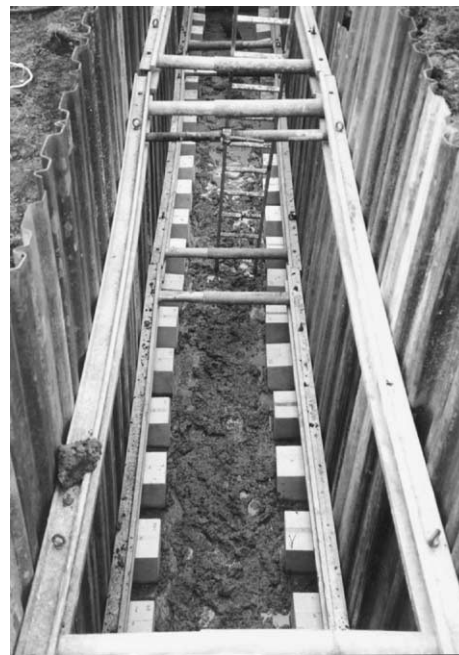
Fig. 1. Precast concrete specimens placed at 2.5 m depth in trial trench, awaiting casting of intermediate cast-in situ cubes in May 1998.
