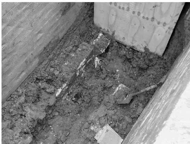
Fig. 2. Removal of concrete specimens from three-year trench in June 2001. White TSA reaction product is clearly visible.
