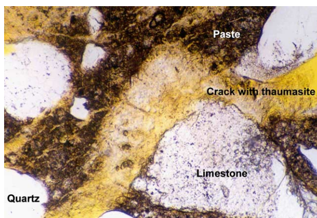
Fig. 4. Crack filled with thaumasite crystals, ≈4 mm below the surface. Photo size 0.6 × 0.9 mm.
