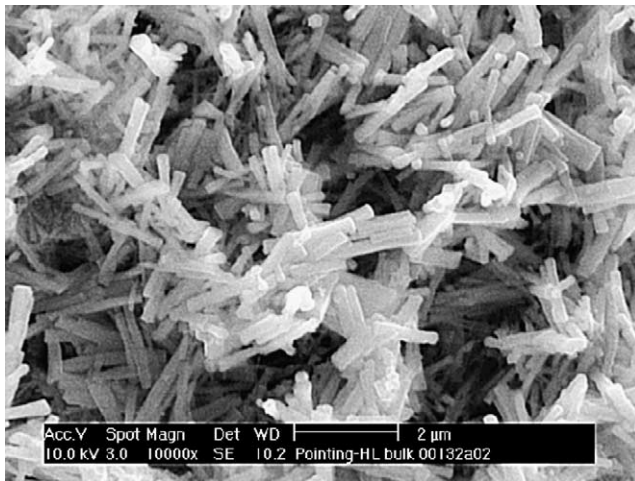
Fig. 13. SEM picture of thaumasite in mortar prism based on hydraulic lime.
