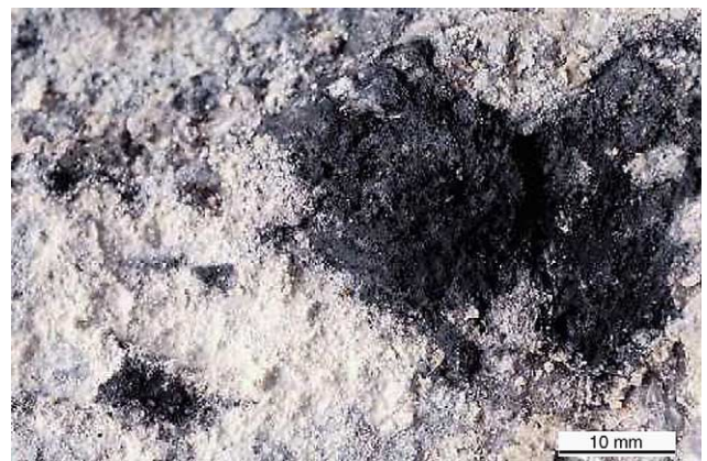
Fig. 4. Surface detail of shotcrete interface to stonework with soot relicts (black) next to soft alteration products (whitish) of the concrete.
