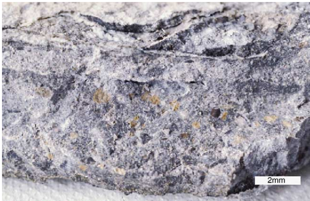
Fig. 2. Fracture surface through shotcrete lining showing several contact parallel bright textures in the shotcrete (tunnel surface at the bottom).
