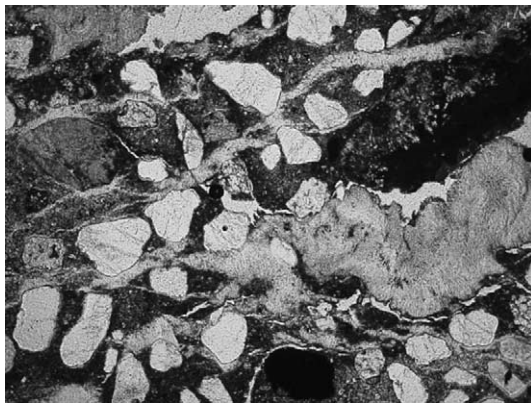
Fig. 6. Zone 3 and 4 TSA development within structural concrete. Thaumasite shown is light yellow coloured, quartz sand grains are white and the remaining cement paste matrix is brown. Image width 4 mm taken in plane polarised light.
