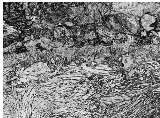
Fig. 3. Natural thaumasite sample showing the interface between the colourless well-formed acicular crystals (bottom) and the straw yellow, finely crystalline, and randomly orientated thaumasite mush typically observed within TSA-affected concretes (top). Magnification \times 33 (PPL).
