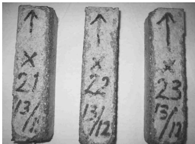
Fig. 2. Storage of mortar prisms with 20% limestone filler (upper) and 20% quartz filler (lower) in 5% sodium sulfate solutions with excess gypsum at 5 °C. Pictures are from the 12 month terminus.
