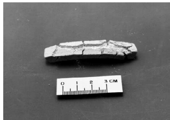
Fig. 4. High alumina type 3 mortar, soaked in water nine months. Mortar broken down through expansion mechanism.
