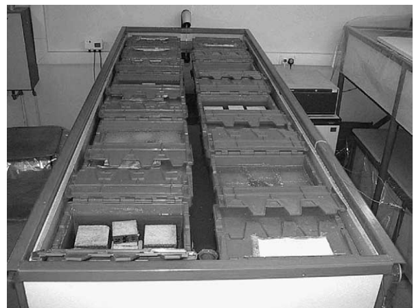
Fig. 1. One of the four sulfate/acid solution exposure tanks maintained at 4.5 °C.
