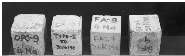
TYPE 1 TYPE V FLY ASH SILICA FUME 4% – Na 2 SO 4 Solution – 24 Months.
