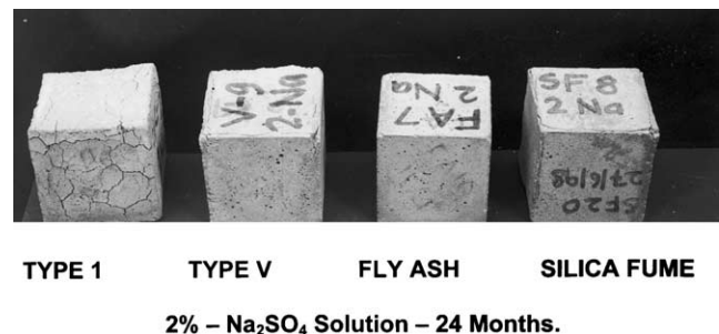
Fig. 3. Plain and blended cement mortar specimens exposed to 2% sulfate solution for 24 months.
