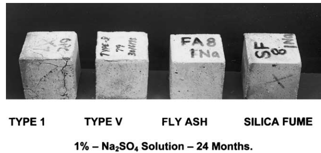
Fig. 1. Plain and blended cement mortar specimens exposed to 1% sulfate solution for 24 months.
