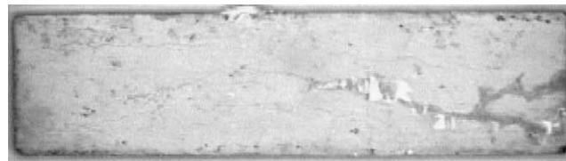
Fig. 17. Exudation of ASR gels on the surfaces of a mortar prism.
