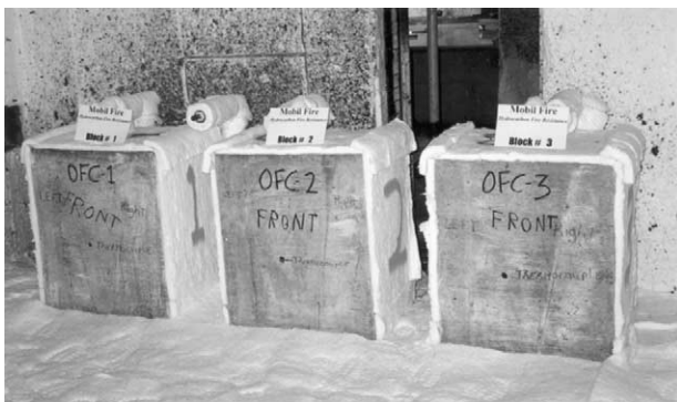
Fig. 2. View of three blocks before the hydrocarbon-fire test.
