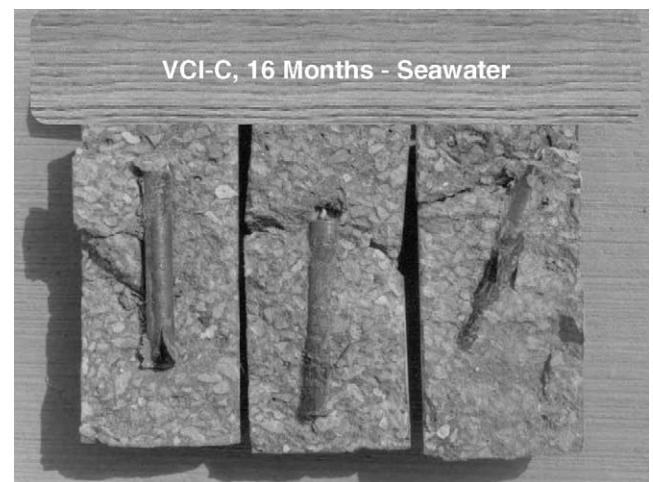
Fig. 10. VCI-C coated rebarred concrete in seawater. Immersion time: 16 months.
