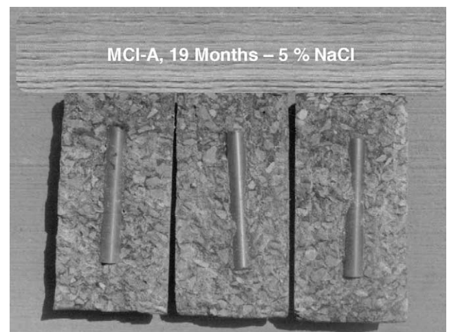
Fig. 9. Rebars in MCI-A coated concrete in 5% NaCl solution. Immersion time: 19 months.
