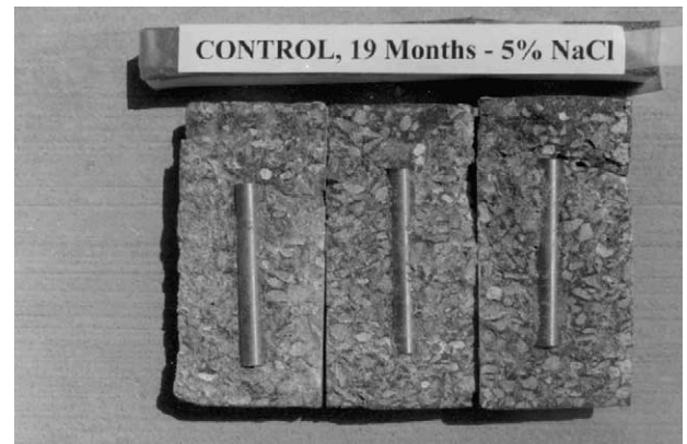
Fig. 8. Rebars in concrete under controlled condition in 5% NaCl solution. Immersion time: 19 months.
