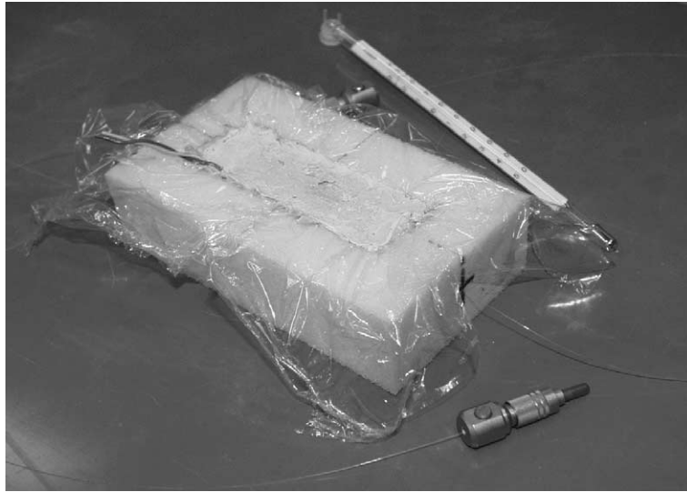
Fig. 2. Cement paste specimen in form, sensor fibre and optical adapters.
