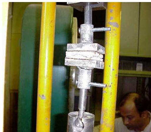
Fig. 5. Internal bond test set-up.
