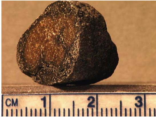
Fig. 1. Nodule of portland cement clinker with a cut and polished face.
