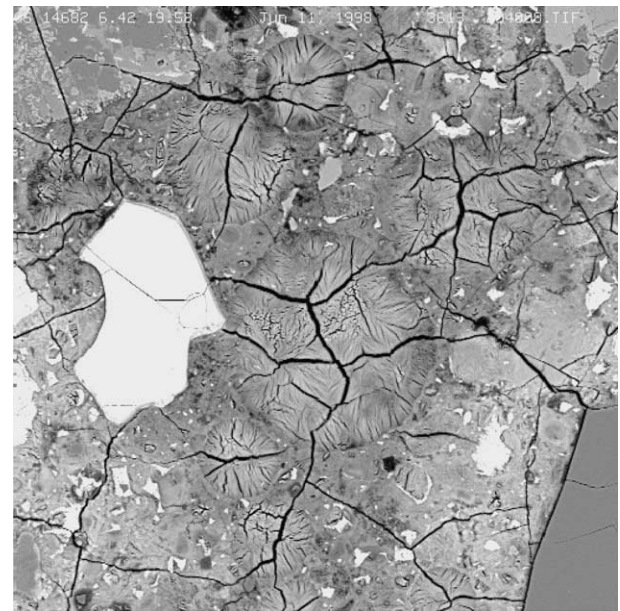
Fig. 16. A region of paste in the Type V concrete in which the air voids are filled. The pattern of cracking appears to be indifferent to these filled voids, passing directly through them.
