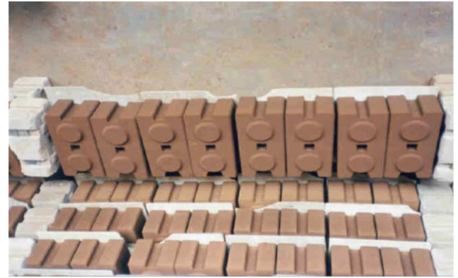
Fig. 1. The shape of commercial soil–cement blocks (0.125×0.25×0.1 m).
