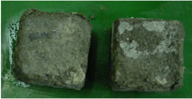
Fig. 4. SF10-45 mortar cubes immersed in 5% magnesium sulfate solution for 510 days.
