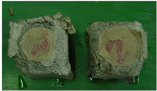
Fig. 1. OPC-45 mortar cubes immersed in 5% sodium sulfate solution for 510 days.
