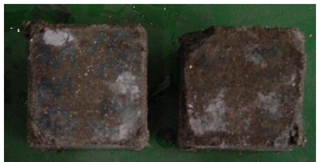
Fig. 3. OPC-45 mortar cubes immersed in 5% magnesium sulfate solution for 510 days.
