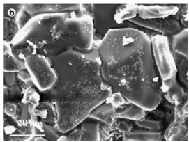
Fig. 2. SEM photos of pure (a) and doped (b) clinker.
