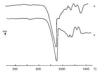
Fig. 1. DSC curves of pure (a) and 2% doped sample (b).
