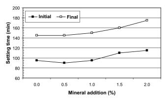
Fig. 4. Setting time of the cements in relation to the percentage of the added mineral.
