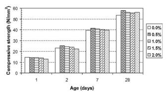
Fig. 3. Strength development of cements in relation to the percentage of the added mineral.
