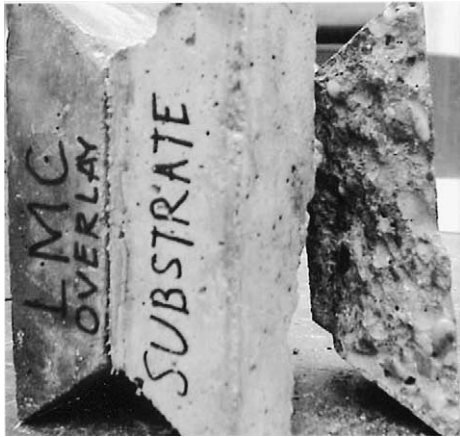
Fig. 9. Typical failure of latex modified concrete bi-layer specimen (substrate failed but interface intact).
