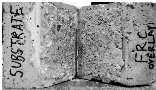
Fig. 12. Typical failure of fiber reinforced concrete bi-layer specimen (failure on substrate side of specimen).
