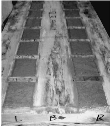
Fig. 2. Substrate specimens cast in partitioned wooden molds.
