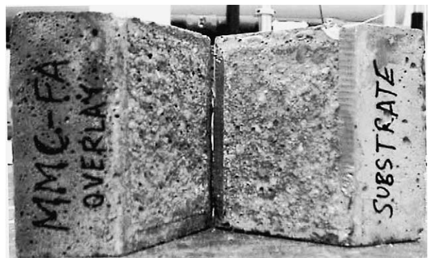
Fig. 11. Typical failure of silica fume-fly ash modified bi-layer specimen (failure on substrate side of specimen).
