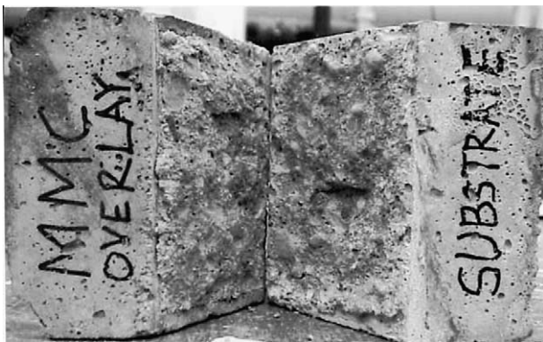
Fig. 10. Typical failure of silica fume modified bi-layer specimen (failure on substrate side of specimen).
