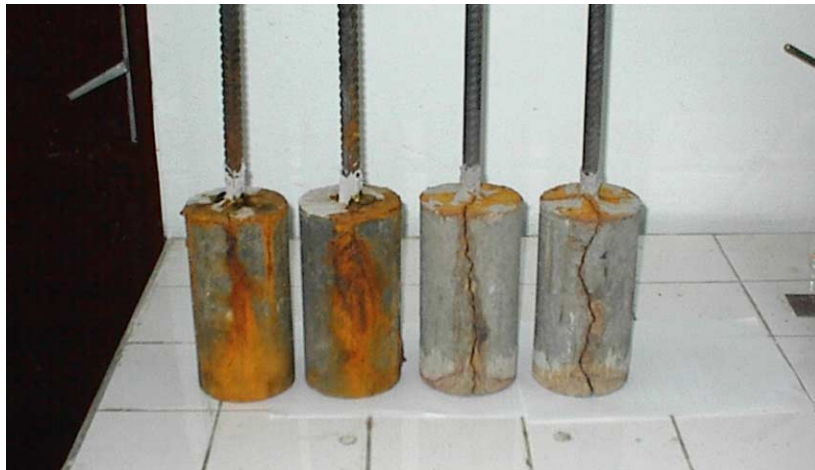
Fig. 8. Typical corrosion specimens after the accelerated corrosion test.
