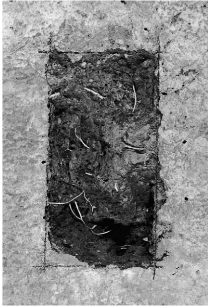
Fig. 9. Soil-cactus pulp slab quantity eroded 40.89 g.
