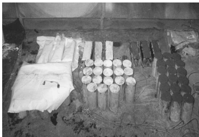
Fig. 1. Test specimens and various curing methods.
